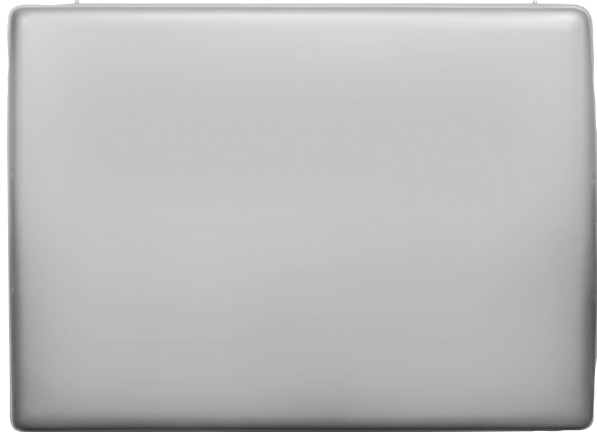
3752WT 1966-77 Roof Panel, Weld Through Primer
