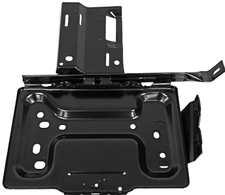
3097A NEW 1987-96 Auxiliary Battery Tray w/ Brace, Diesel, LH
